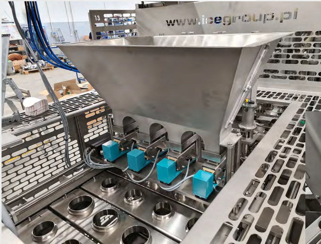
Electric vibrators with individual lane control
