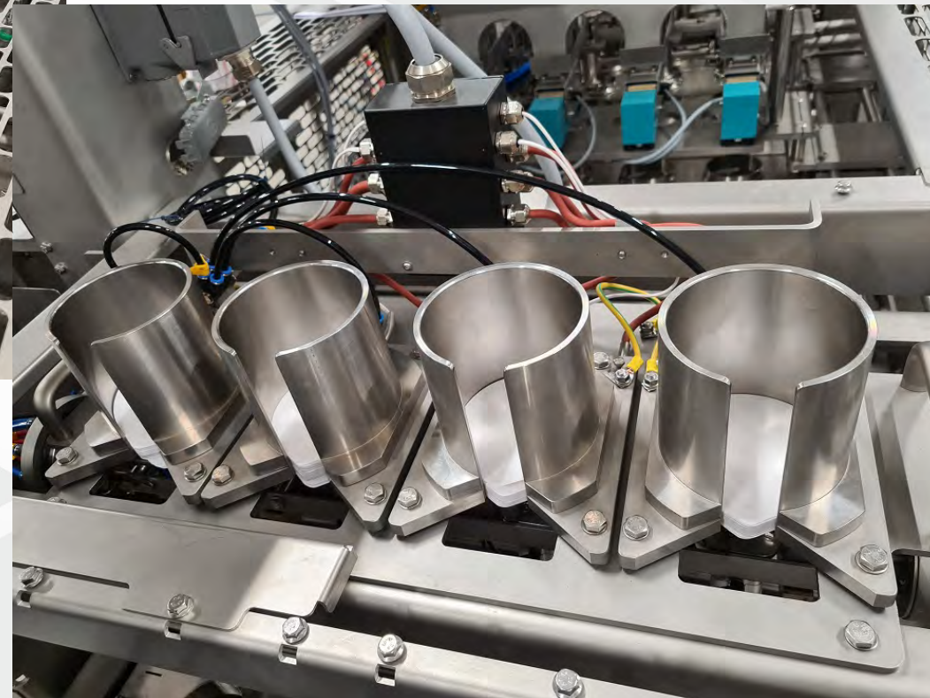
Heated sealing lids magazines with individual lane control
