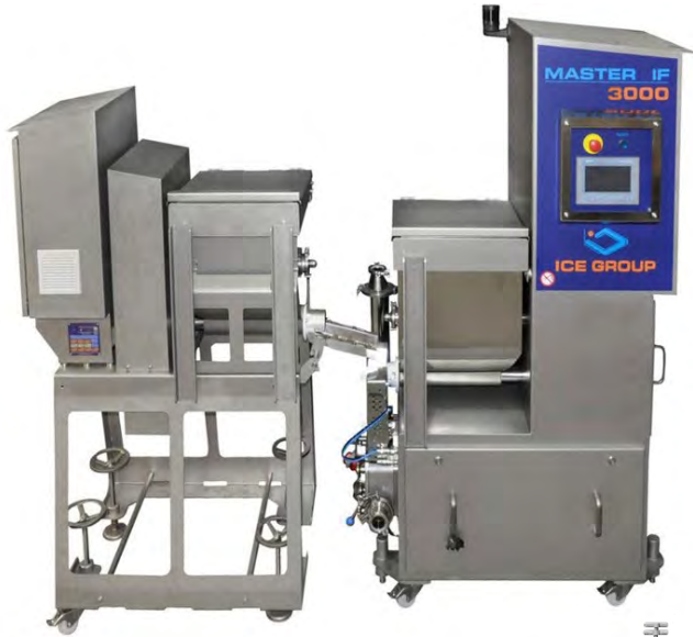
Master IF 3000 fruit feeder with CCF (Constant Crispies Feeder)
