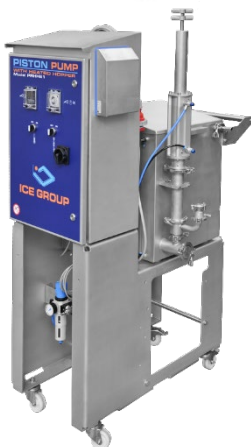
One piston pump for syrup or chocolate with heated hopper
