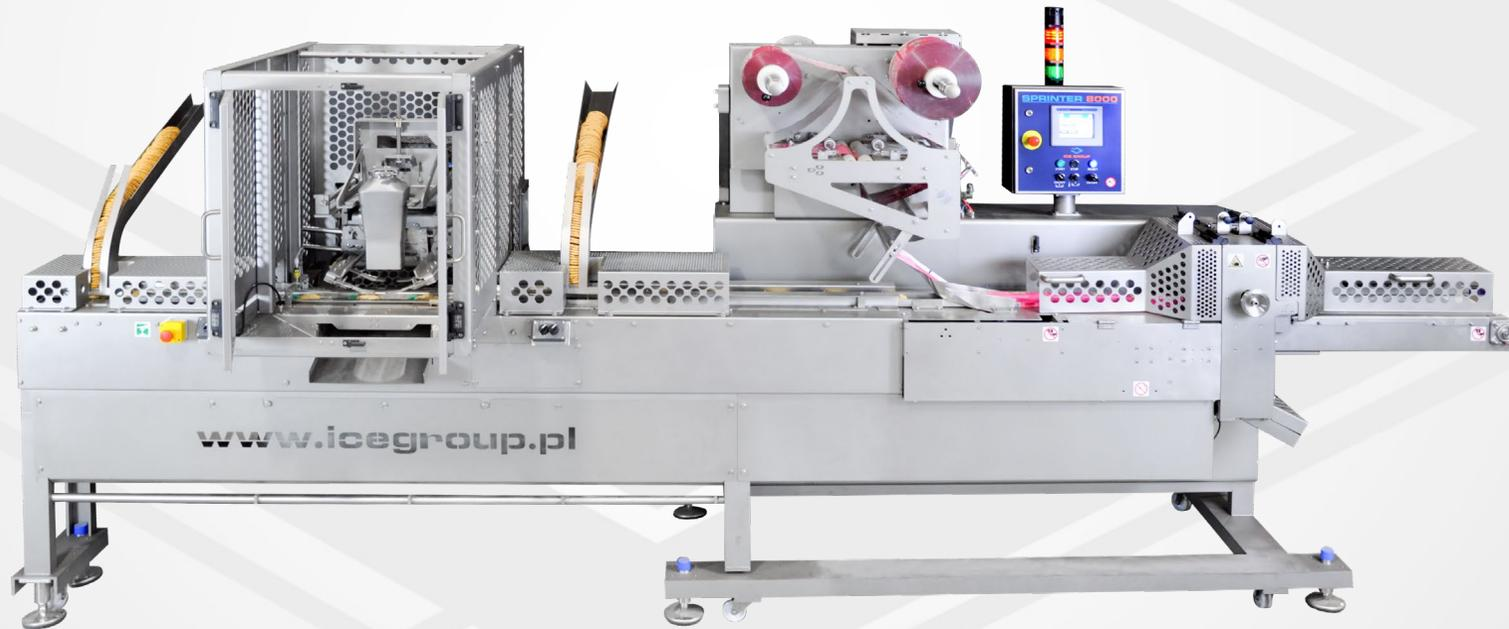
Sprinter is an independent ice cream sandwich production machine, constituting an extension of Rapid Servo flow-pack machine. In case of our Special Sprinter machine, apart from the classical two-arm servo-driven extruding and cutting station, we have a second exchangeable servo-driven, follow-up dosing station on a movable frame, which can be used for work with large solid pieces.
